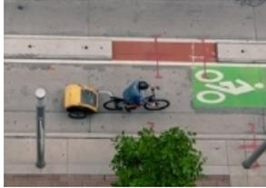
Bike lanes that are physically separated from vehicle traffic and parking lanes using vertical and horizontal features, such as bollards, planters, and parked vehicles.
