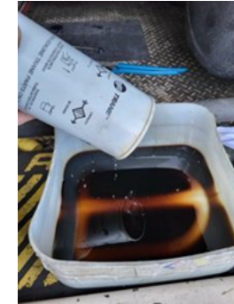
Photos of the circuit 1 very dark oil and oil sample analysis results
