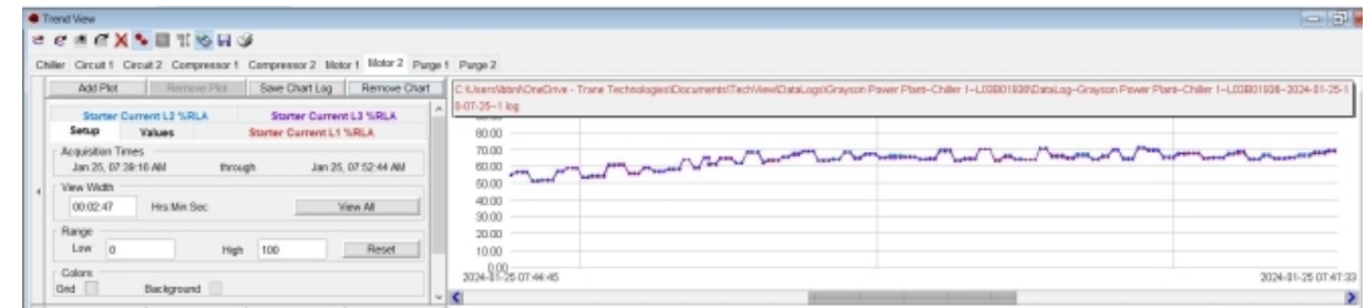
Photo of circuit 2 testing showing erratic amperage fluctuations
